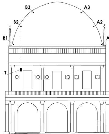
Fig. 1. Schematic cross section of the “Palazzo della Loggia” with the indication of the symmetric points A1-B1, A2-B2, A3-B3, in the wooden vaulted roof, where the couples of iron and invar wires were stretched. The possible positions of the “muon telescope” (T), linked to a structural element of the building (the fixed reference system), and the “muon target”, connected on a point of the roof to be monitored, are shown.
