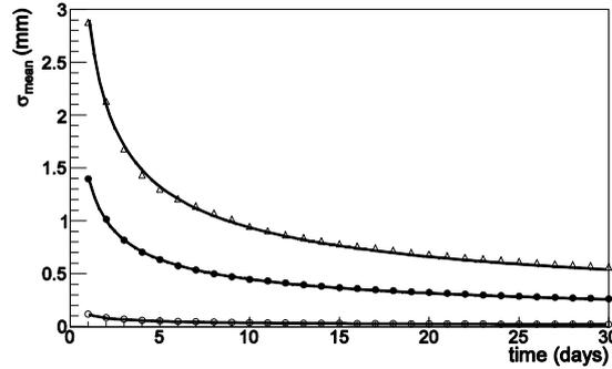
Fig. 4. Standard uncertainty on the mean value of the  $\Delta x$  sample distributions versus data taking time, for the “muon target” in position B1 (open circles), B2 (full squares) and B3 (open triangles). Fitting curves are given by the general relation  $\sigma_{mean} = C/\sqrt{t}$ ;  $C$  is a constant and  $t$  is the data taking time.
