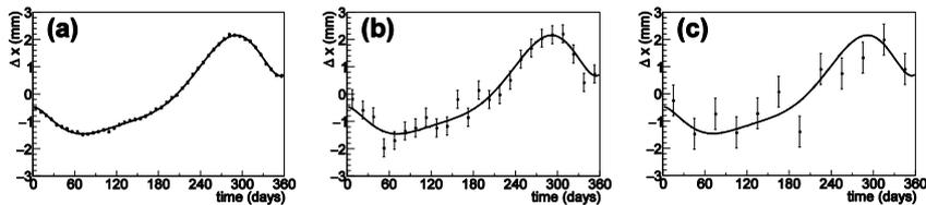
Fig. 5. The same seasonal deformation corresponding to the first year of data taking in Fig. 2, with superimposed the result of the simulated measurements of the position of the “muon target”, displaced following the assumed structure deformation. Sampling rate is one week for position B1 (a), two weeks for position B2 (b) and one month for position B3 (c).
