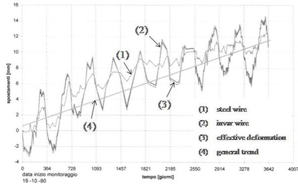
Fig. 2. Elongation of the wires stretched between the points A2 - B2 of the truss wooden arch as a function of time in days. Ordinary steel wire (1), invar wire (2), effective deformation of the structure after accounting for the thermal elongation of the wires (3), general trend of deformation (4). (Courtesy of the authors of Ref. 19)
