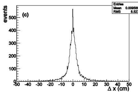
Fig. 3. Distributions of the difference  $\Delta x$  between the crossing point coordinates measured on the “muon target” in position B3, and the crossing point coordinates of the linear extrapolation of the muon trajectory measured by the “muon telescope”, with 15.0 cm thick wooden floor interposed. Simulated data taking time is 15 days.
