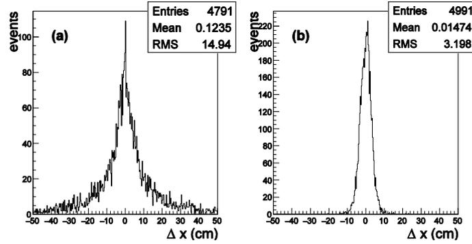
Fig. 6. Distributions of the statistical variable  $\Delta x$  for the position B3, with one 30.0 cm thick concrete floor interposed and data taking time of 7 days, in the case of straight (a) and broken (b) line models.
