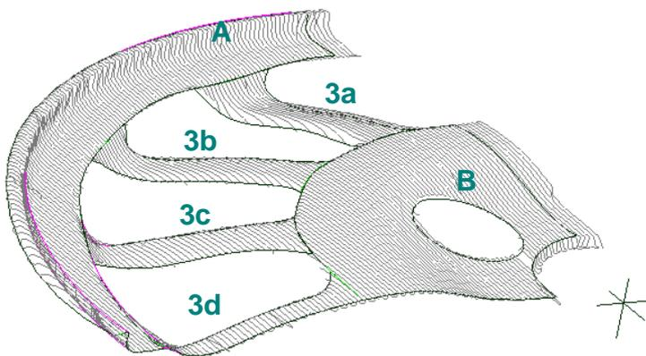
Figure 8: NURBS surfaces of the 'rough' CAD model
