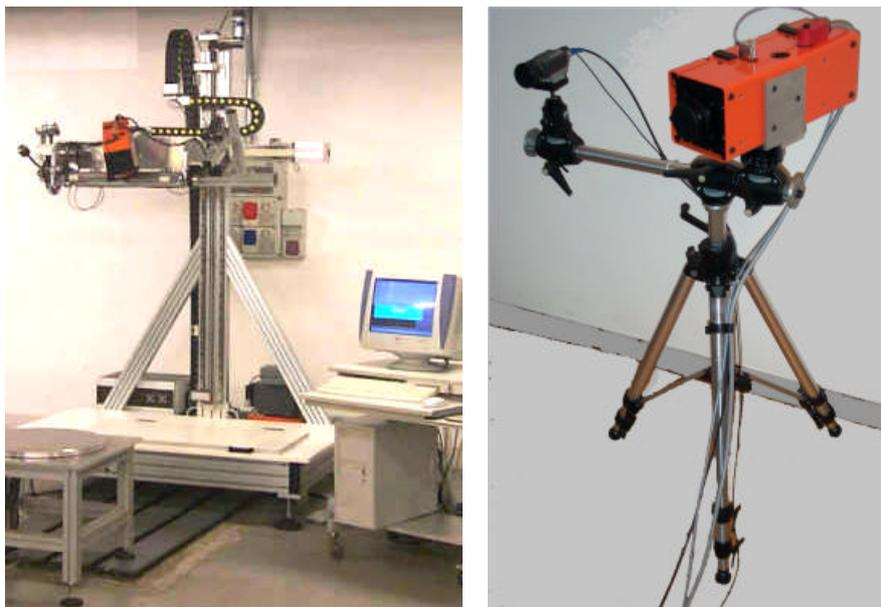
Figure 3. Prototypes used for the contactless digitization of the surfaces
