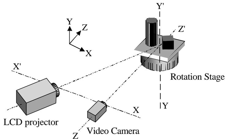
Figure 2. Optical geometry of the 3D vision system
