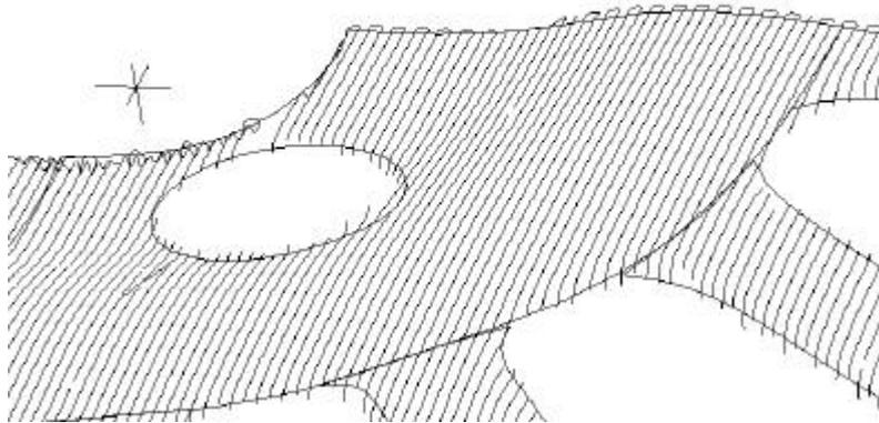
Figure 7. Scan curves and boundary curves defined by PRO/E
