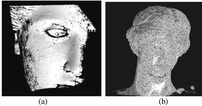
Figure 3. Point cloud acquisition of the “Vittoria Alata”. 3.a: single point cloud corresponding to the right side of the face of the statue; 3.b: result of the alignment of 41 view of the head.
