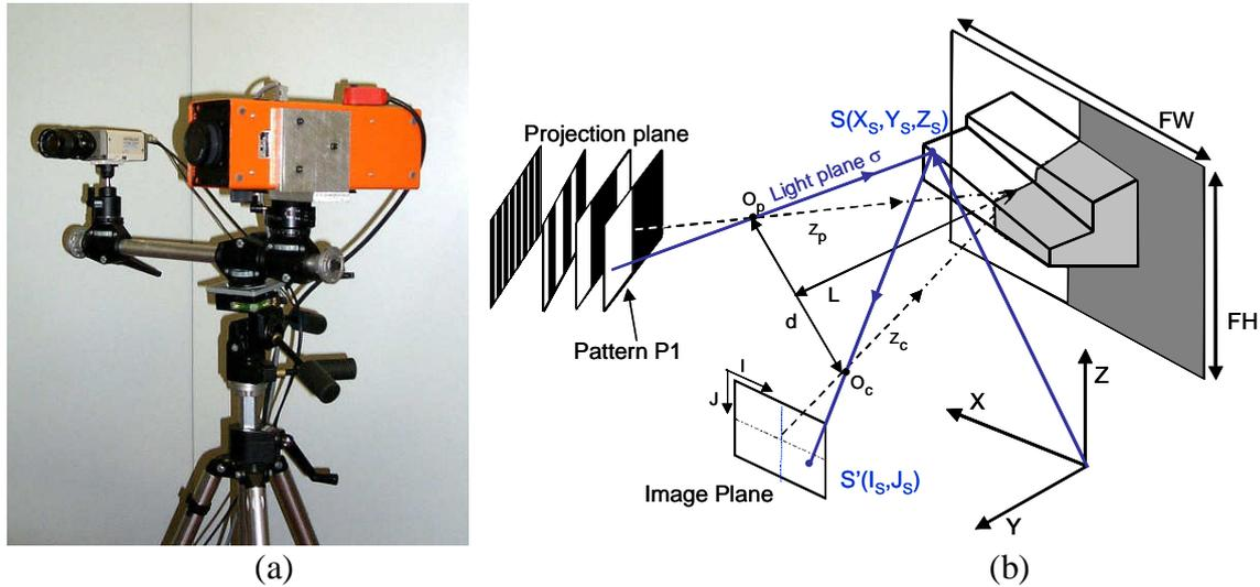
Figure 2. The optical digitiser OPL-3D. a: image of the instrument; b: optical layout.
