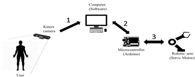
Figure 1. Scheme of the remote control System
