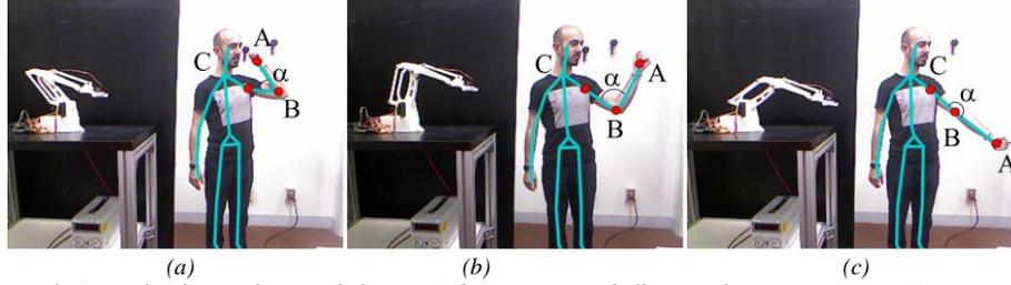
Figure 3: Example of control system behavior. Robot position and elbow angle computation at (a) minimum, (b) middle, and (c) maximum arm position.
